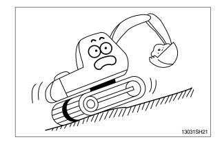
Operate the machine after making ground flat when operation is required on a slope.
