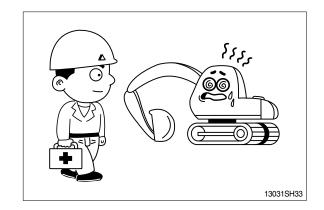
Park on a flat place and stop the engine for inspecting and repairing. Properly TAG machine is not operational. (Remove start key) Extreme care shall be taken during maintenance work. Parts may require additional safe guard.
